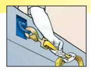
FROM YELLOW WEBBING SIDE OF BRACE, ATTACH HOOK TO THE BRACKET RING.
