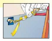
LOOP THE RED WEBBING AND HOOK AROUND LADDER SIDE RAIL AND CLIP TWIST HOOK TO FYF RING.
