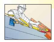
TIGHTEN BELT BY **PULLING YELLOW** ADJUSTING BELT
